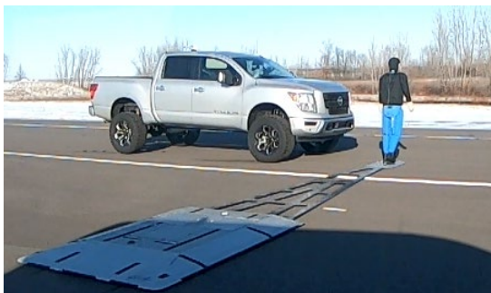
FIGURE 8B . P-AEB TEST PHOTO (ADULT TEST CPNA)
