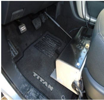
FIGURE 7. THROTTLE ROBOT, INTERIOR CAMERA AND GPS NAVIGATION
