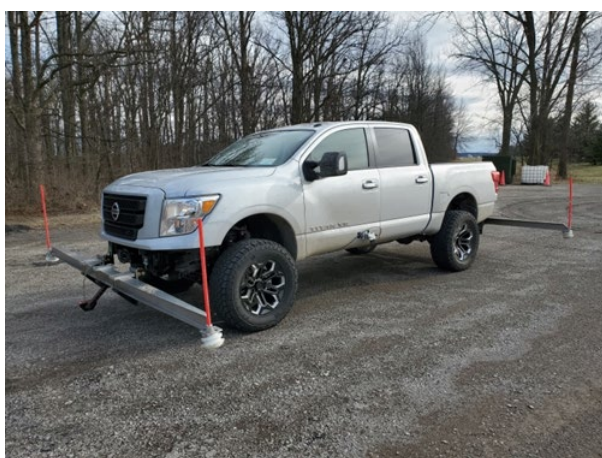
FIGURE 15. FMVSS 126 INSTRUMENTATION – OUTRIGGERS AND STEERING ROBOT
