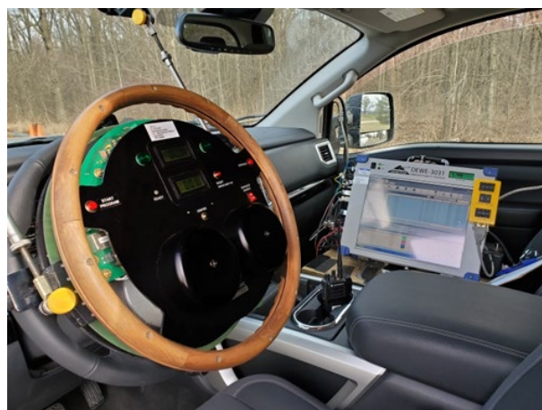
FIGURE 15. FMVSS 126 INSTRUMENTATION – OUTRIGGERS AND STEERING ROBOT
